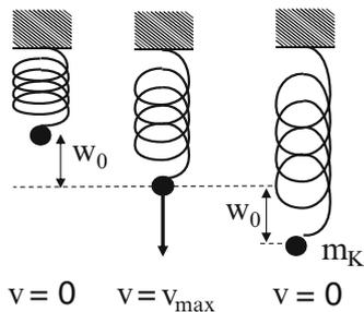
**Fig. 63** Vibrating spring loaded with a mass
