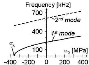
**Fig. 72** Resonance frequencies of a vibrating beam as a function of residual stress calculated with (170) and (161)
