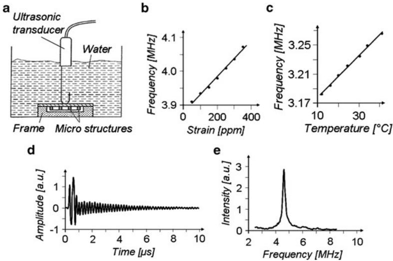
**Fig. 62** Experimental test setup for micromembrane sensors [39] (a); Measured resonance frequency as a function of strain (b) and temperature (c); Measured signal from the micromembranes (d); and Fourier transformation of the second part of that signal (e). (Courtesy of Karlsruhe Institute of Technology, KIT)
