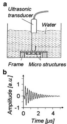
**Fig. 68** Micromembrane sensor with an open frame (a) and signal measured with this sensor (b)
