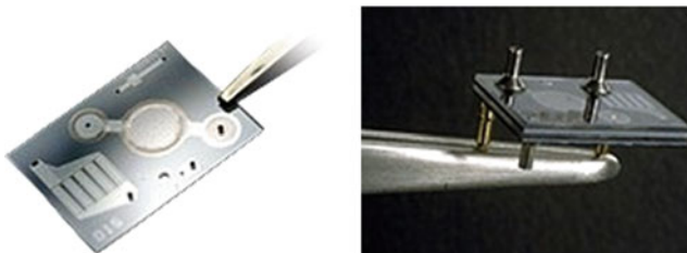
Fig. E31 Implantable micropump [69] (Courtesy of Debiotech SA/Switzerland)
