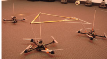
Fig. 3 The aerial robots and manipulation payload for experimentation. The payload is defined by m = 0.25\text{kg} and \bar{x}_2^p = 1\text{m} , \bar{x}_3^p = 0.5\text{m} , and \bar{y}_3^p = 0.87\text{m} , with l_i = 1\text{m} .
