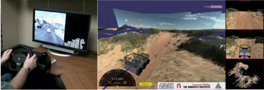
Fig. 6 OCS. The Operator Control Station includes a steering wheel equipped with selection buttons, foot pedals, and a large LCD display. The display provides selectable views including the raw video, over-the-shoulder, and birds-eye (direct overhead). The selected view is enlarged and the others are reduced in size and shown to the right.
