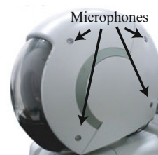
Fig. 5 ASIMO has two pair of 4 mics on each side.
