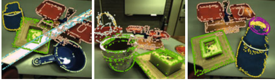
Fig. 9 Cluttered scenes with pose estimates. Local features of object models are back-projected into the image at the estimated pose; false colors identify different objects.
