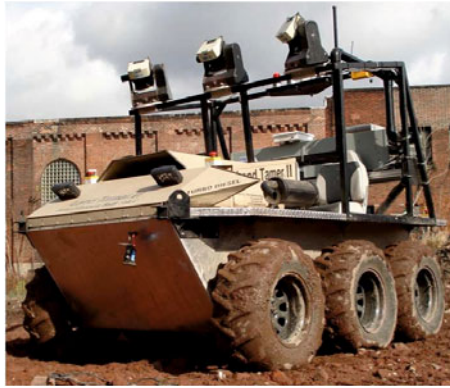
Fig. 5 Robot Vehicle. A LandTamer® vehicle was retrofitted for remote control. Three custom colorized range (CR) sensors with a total field of view of 160^\circ are mounted high on the vehicle looking forward. The lidars are manufactured by SICK providing range points at 2 KHz separated by \frac{1}{2} degree of angle over 180^\circ of field of view. The cameras are the Firefly® by Pt. Grey Research Inc., and they provide color imagery at 720 X 500 resolution over a 60^\circ field of view.
