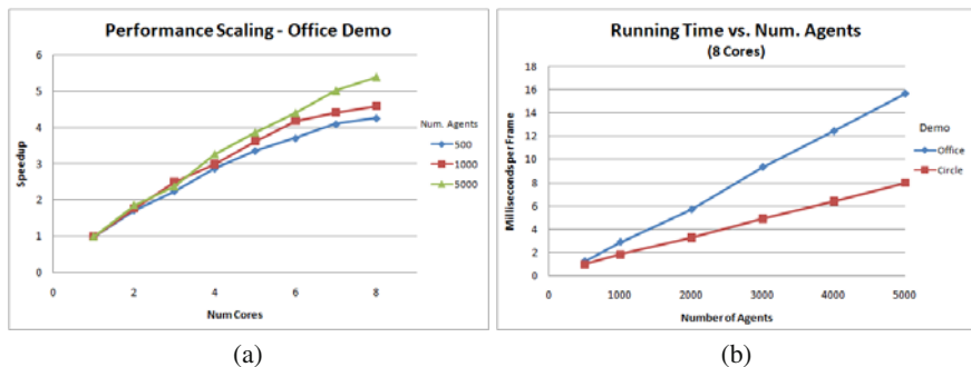
Fig. 10 Performance Graphs: (a) Performance scaling on the evacuation simulation for 1 to 8 cores. (b) Runtime for various number of agents on 8 cores (lower is better). Both simulations scale approximately linearly with the number of agents.
