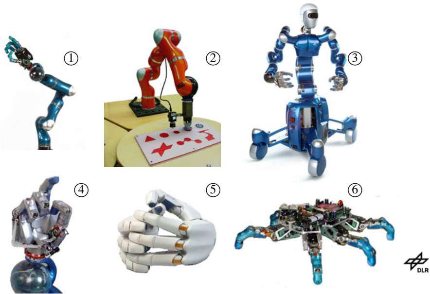
Fig. 1 Overview of the DLR Robots: ①: The DLR-LWR III equipped with the DLR-Hand II. ②: The DLR-KUKA-LWR III which is based on the DLR-LWR III. ③: The DLR Humanoid “Rollin’ Justin”. ④: The DLR-Hand II-b, a redesign of the DLR-Hand II. ⑤: The Schunk Hand, a commercialized version of the DLR-Hand II. ⑥: The DLR-Crawler, a walking robot based on the fingers of the DLR-Hand II.
