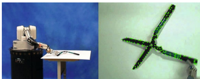
Fig. 1 UMan (UMass Mobile Manipulator) performs a manipulation task without prior knowledge about the manipulated object. The right image shows the scene as seen by the robot through an overhead camera; dots mark tracked visual features.
