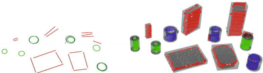
Fig. 12 A slightly different reconstruction of the scene presented previously in Figure 9. Left: the 2D shapes that were fit to the cluster. Right: the inliers of those shapes in 3D.
