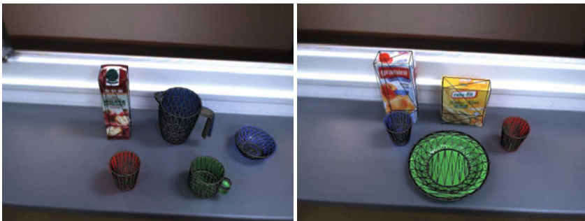
Fig. 2 Exemplary results with the integrated proposed object recognition and pose estimation systems. The computed object pose has been applied to the 3D object model and the wireframe model has been overlaid.
