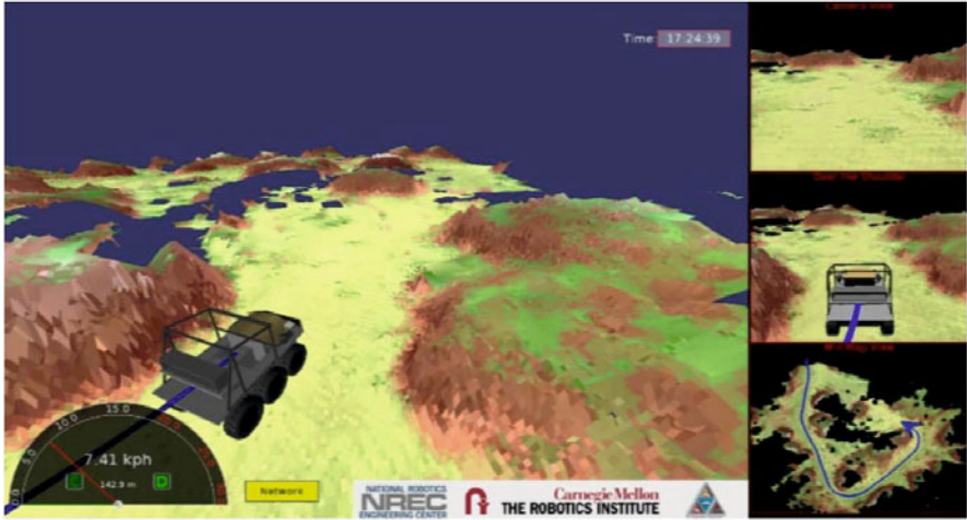
Fig. 9 Augmented Reality Display for Autonomy Assisted Hazard Avoidance. The photo-realistic display is augmented with false color obstacle annotations. Billboards are turned off.
