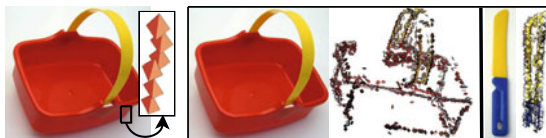
Fig. 7 ECV descriptors. Left: ECV descriptors are oriented appearance patches extracted along contours. Right: object-segmented and refined ECV descriptors via structure from motion.
