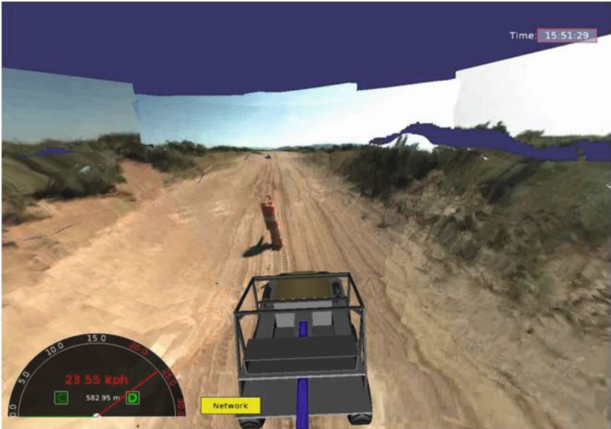
Fig. 10 High Speed Obstacle Avoidance. Latency compensation is most valuable during high speed driving. Here, the operator avoids an obstacle to the right, fitting the vehicle into a narrow space. A custom fly-behind view was used. The speedometer reads 24.55 km/hr. The operator control station is about 1 km further down the road.
