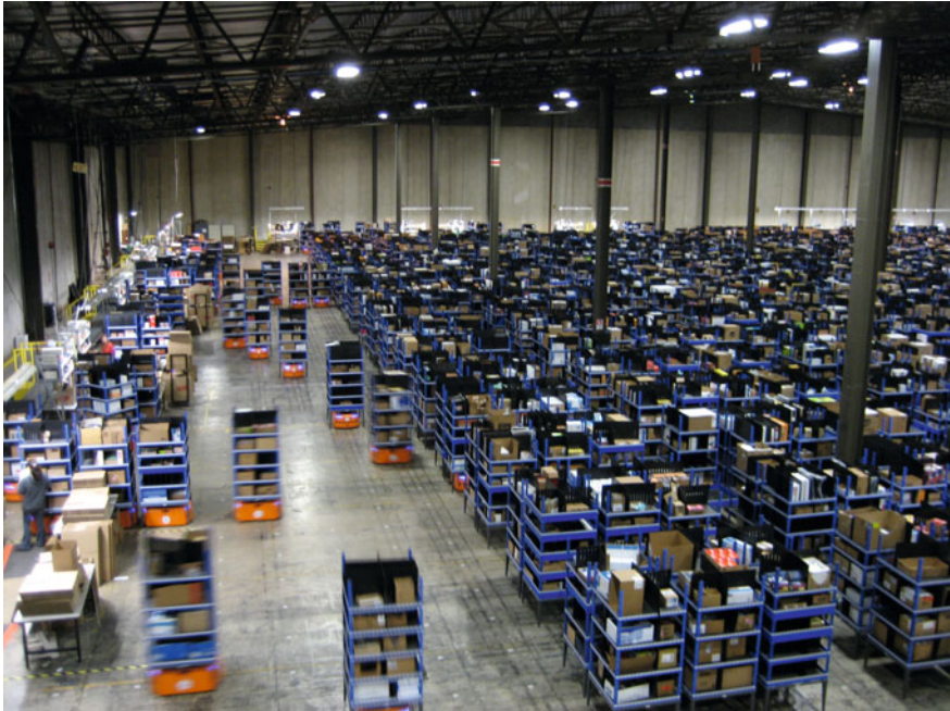
Fig. 1 A Kiva warehouse. The blue shelves hold the inventory and can be moved by the robots. The workers stay at fixed stations and the robots move around the warehouse to pick up the inventories and bring them to the stations. The underlying navigation grid can be inferred from the marks left by the robot wheels.
