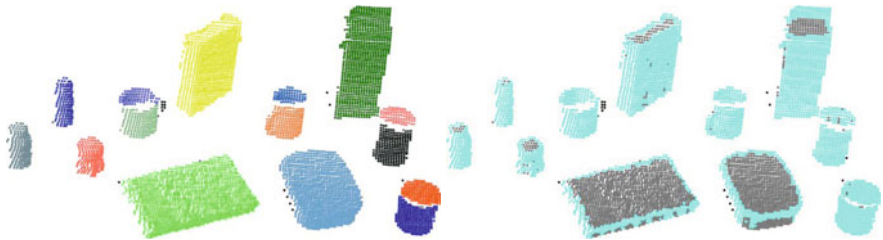
Fig. 5 Left: the identified objects on the table based on the clustering of their projections shown in random colors. Right: points that lie on the boundaries of the clusters are highlighted.
