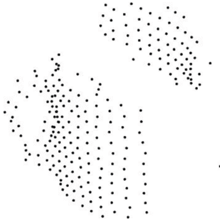
Fig. 2 Typical one-side scan of a mug, where the rim and handle didn't return enough measurement points, thus the mug will be over-segmented into two separate connected components, and the handle is hard to detect.
