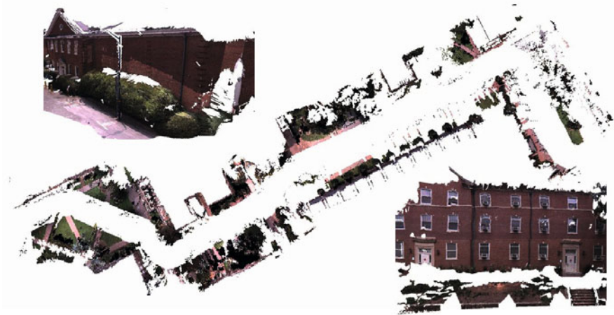
Fig. 10 Top view of segment of the Chapel Hill reconstruction with two views of facades.
