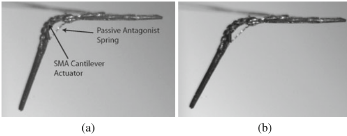
Fig. 6 HAMR's leg a) unactuated and b) actuated to maximum displacement. The maximum measured angle was 9.1 degrees.
