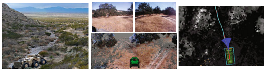
Fig. 1 Left: The Crusher platform is capable of long range autonomous navigation through complex terrain. Center: Raw perception data from Crusher, in the form of camera images and colored LiDAR. Right: 2D costs derived from perception data. Brighter pixels indicate higher cost.
