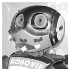
Fig. 4 Robovie R2 has 8 mics around its head.
