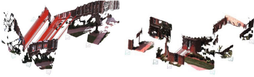
Fig. 14 3D registration of 2 3D models with 45° viewing direction change using VIP features.
