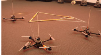
Fig. 3 The aerial robots and manipulation payload for experimentation. The payload is defined by m = 0.25 kg and \bar{x}_2^p = 1 m, \bar{x}_3^p = 0.5 m, and \bar{y}_3^p = 0.87 m, with l_i = 1 m.
