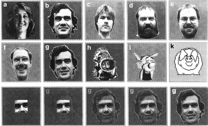
Fig. 4.7 Pattern recognition of faces by means of the synergetic computer. Top : examples of prototype patterns stored in the computer, with family names encoded by letters. Bottom : when part of a face is used as an initial condition for the pattern recognition equations, their solution yields the complete face with the family name
