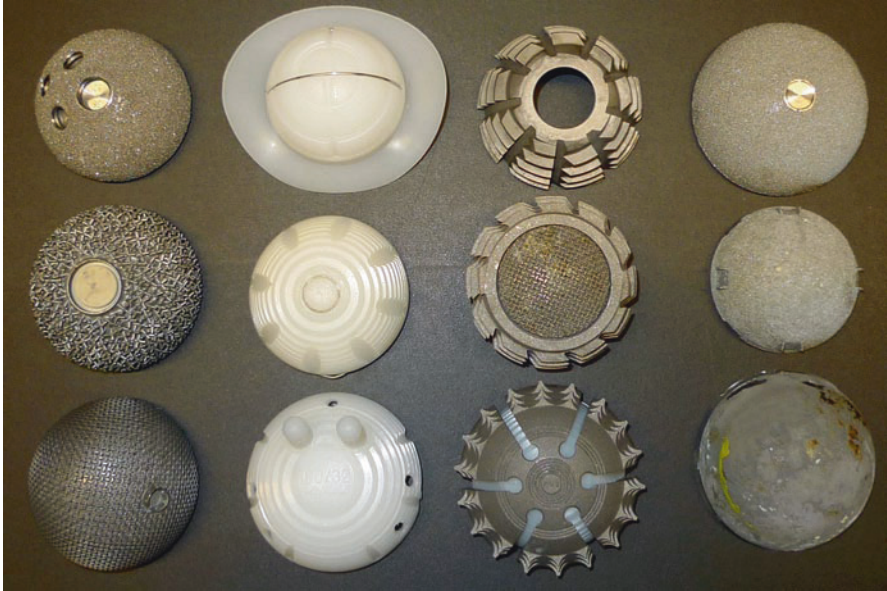
Fig. 2.3 View of the backside of new and revised acetabular components; from left to right ( columns ): press-fit uncemented cups, cemented cups, threaded ( bottom : expansion) cups, monobloc cups
