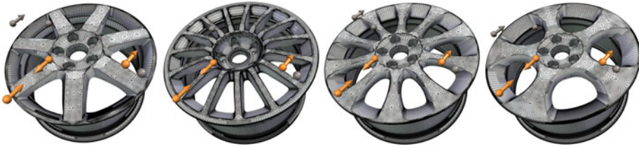
Fig. 3. Three classes of car rims. The spokes of the three rims types are generated by different 'overriding' functions. Right image: Changing the number of spokes.
