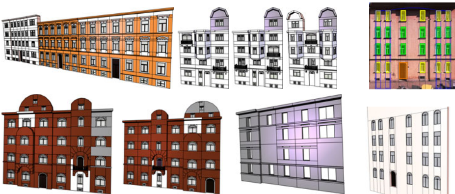
Fig. 7. CITYFIT examples. A GML shape grammar for Convex Polyhedra is generated automatically from the results of an image analysis pass (images to the right).
