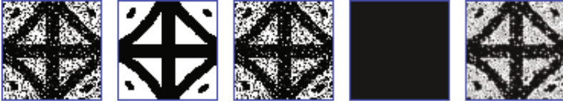
Fig. 2. Exemplar result of binary synthetic image denoising. From left to right: disturbed image, ground-truth and columns 3-5 are regression results of \varepsilon -SVR, \text{SSVR}^{cube} and our SSVR. Values lower than 0 or higher than 1 are adjusted to 0 or 1 respectively.
