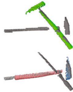
Fig. 4. Example pose estimates. Grey dots correspond to scene points; color dots show object points aligned to the scene through pose estimation. The single-part model fails to produce a correct estimate (top), whereas a two-part model succeeds (bottom).
