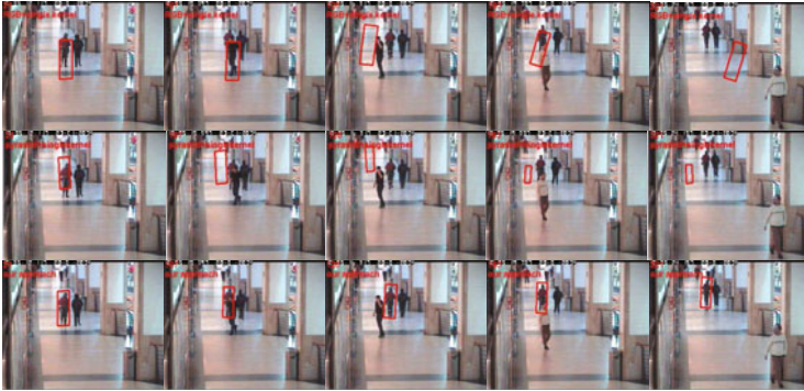
Fig. 6. “EnterExitCrossingPaths1cor”sequence Top row: results of RGBSVM. Middle row: results of pyramidSVM. Bottom row: results of our approach.
