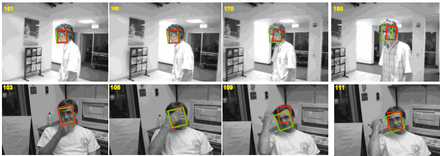
Fig. 3. Comparison of filter distraction and partial occlusion handling (red box: IVT, green box: proposed method via the layered sampling, row 1: 'daivd' and row 2: 'dudek' sequences)
