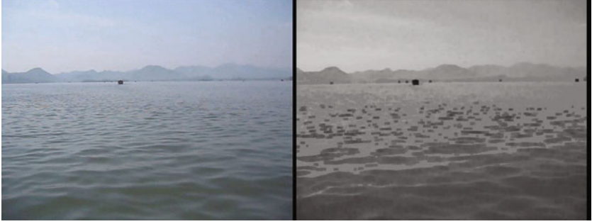
Fig. 1. Left: input image. Right: the dark channel image with 5 \times 5 rectangular kernels.
