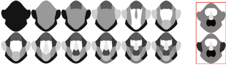
Fig. 3. Facial components found by applying the k-means++ clustering algorithm to the similarity features described in Section 3. The features were computed on the 3D shape of a dataset of 187 registered laser scans of the human face. The red box ( right ) shows manual segmentations of the face into four and five regions as used in our experiments (Section 5.1). The manual subdivisions correspond well with those commonly found in the literature.
