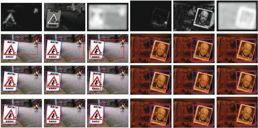
Fig. 3. Detection results comparison among our MSD, exhaustive search and MSR. The first row are two examples of saliency maps for Hou’s [7], Achanta’s [12] and Bruce’s [9] methods respectively. The second row are localization results by exhaustive search on the three saliency maps. The third row are results by MSR. And the last row are our MSD results. Detected results are labeled with bold red line. Blue plain rectangles are ground truth from [4].
