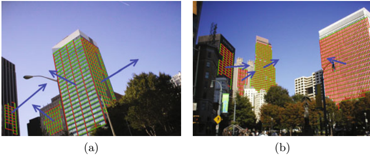
Fig. 12. This figure shows the computation of surface normals from a lattice detected on a building facade. The blue arrow indicates the surface normal of the building.
