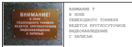
Fig. 2. Text localization and recognition output example on Russian text. Note: The only adjustment of the proposed method was a use of synthetic cyrillic fonts to train the character recognition with a Russian language model. The recognition is error free, with the exception of the exclamation mark which is not included in the training set.
