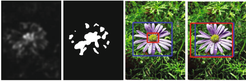
Fig. 1. Our salient object detection result based on the saliency map proposed in [7] (The first image is the saliency map by [7]. The second image is the binarized result of the saliency map. The third image is the result of salient object detection by searching method in [8]. The red bold rectangle is the detected result while the blue plain one is the ground truth from [4]. The last one is the result by our MSD detection method.).
