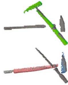
Fig. 4. Example pose estimates. Grey dots correspond to scene points; color dots show object points aligned to the scene through pose estimation. The single-part model fails to produce a correct estimate (top), whereas a two-part model succeeds (bottom).
