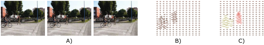
Fig. 1. An illustration of moving object detection from a perspective of optical flow analysis. A) : A video sequence with both object motions and camera motion. B) : The corresponding optical flow. C) : The segmentation result that detects the moving objects.
