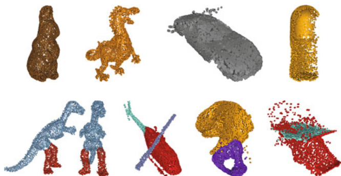
Fig. 7. Object points obtained from the registration of sequences of 66 views. Color indicates learned parts; objects on the first row are made up of a single part, whereas those on the second row yield two- or three-part models. The models of the deodorant bottle (top-right) and of the pedal (bottom-right) were not correctly constructed, because of symmetries and similarities within the objects.
