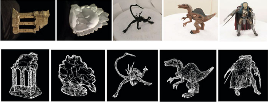
Fig. 4. Input datasets. From left to right: temple, dino, alien, dinosaur, and predator. (top) a sample input image from each dataset, (bottom) reconstructions of the proposed method in a surface-based approach.
