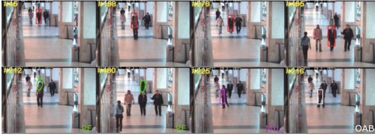
Fig. 2. Comparison of tracking results when there is occlusion. Top row shows results of our approach. Results of other approaches are shown in the bottom row.
