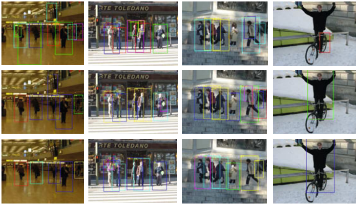
Fig. 8. Some examples of detections on test images for the detectors using PHOG, pyramid uniform CS-LBP and augmented features (combined with HOG and pyramid uniform CS-LBP). First row: detected by the PHOG based detector. Second row: detected by the pyramid uniform CS-LBP based detector. Third row: detected by the PHOG+pyramid uniform CS-LBP based detector.
