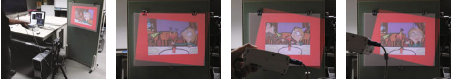
Fig. 1. From left to right: Overview of the projector-camera system. Example of unrectified images. Results obtained by our method; correctly rectified video images are being projected independently of the projector pose. The calibration is automatically performed while a video is projected from the hand-held projector.
