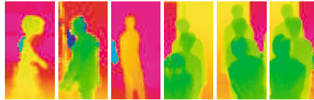
(b) Example of missed detection during classification using depth histogram features (variable of rectangular size)
