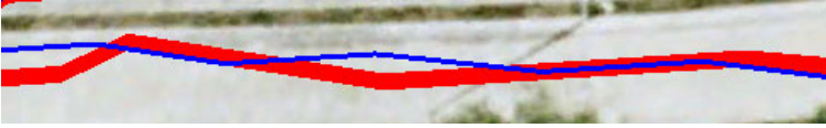
Fig. 5. The reconstruction performance of AACAT on Fleck 3b platform. The thick line is the ground truth and the thin line is the trajectory approximation produced by AACAT. ADE is 3.67 meters.
