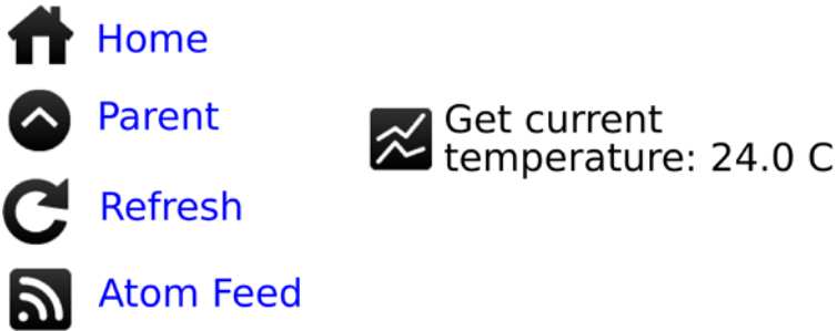
Fig. 5.1b HTML Representation (Rendered by a Browser) of the Temperature Resource of a Sun SPOT Containing Links to Parent and Related Resources
