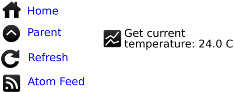
Fig. 5.1b HTML Representation (Rendered by a Browser) of the Temperature Resource of a Sun SPOT Containing Links to Parent and Related Resources
