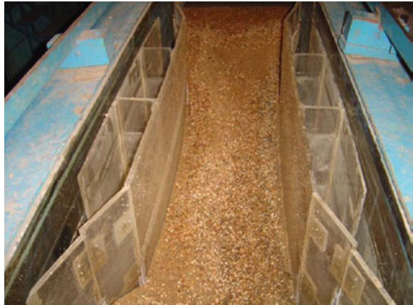
Fig. 10.2 Photograph showing an equilibrium scoured bed within a channel contraction
