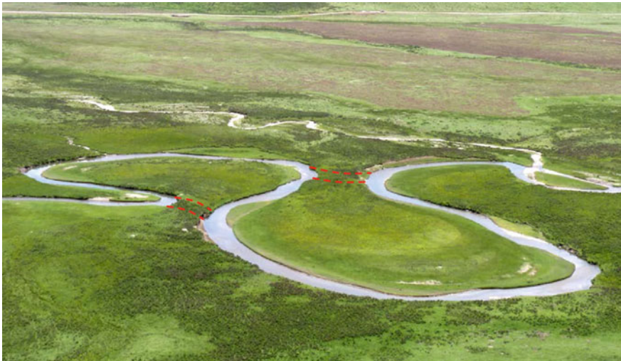
Fig. 9.9 Photograph of the meandering loops of a river showing the potentiality of cutoff by the broken line (courtesy of Z. Wang, Tsinghua University, China)
