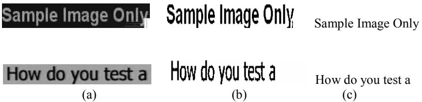
Fig. 4. (a) Image with ROIs identified (b) Binarized text block (c) OCR output
