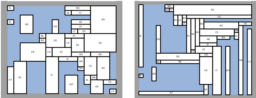
Fig. 2. Two different rectangular duals of the dual graph of a map of Europe. Luxembourg and Moldavia have been removed and “sea regions” have been added to ensure that the dual graph is an irreducible triangulation.
