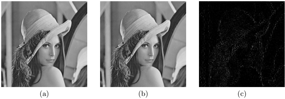
Fig. 4. (a) Original Lena image. (b) Fingerprinted Lena image. (c) Corresponding difference image (amplified by a factor of 10).
