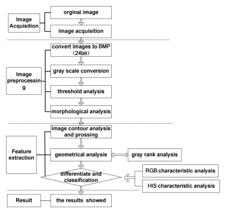
Fig. 2. Detection flowing chart of agricultural products' dimensions
