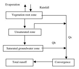
Fig. 1. Structure frame diagram of TOPMODEL
