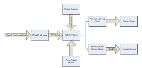
Fig. 1. Hardware Structural of Controller
