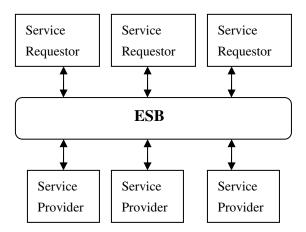
Fig. 3. Enterprise Service Bus Concept model
