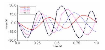
Fig. 7. The reaction of crankshaft bearing on Y axis direction
