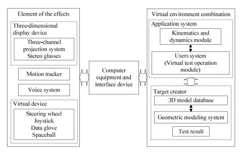
Fig. 1. Structural framework of virtual experiment system
