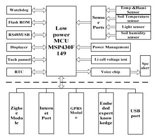
Fig. 2. Structure of hardware
