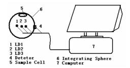
Fig. 2. Structure diagram of the integrating sphere type NIR moisture determination instrument
