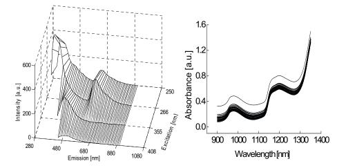
**Fig. 1.** (a) The mean excitation-emission matrix (EEM) for fresh juice; (b) The NIR transmission spectra of the 30 original fresh juice samples. Absorption was calculated by log (I/I0) from transmittance readings.
