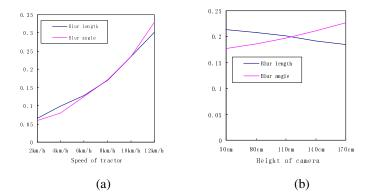
Fig. 4. The trend of tractor speeds and camera height with blurring length and angle
