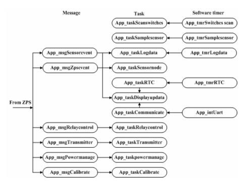
Fig. 4. Software structure
