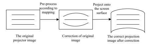
Fig. 5. Schematic diagram of image geometric calibration
