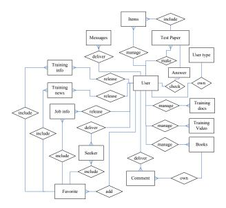
Fig. 3. The E-R diagram of the remote labor training system for rural small town
