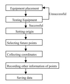
Fig. 3. Flow chart of measurement
