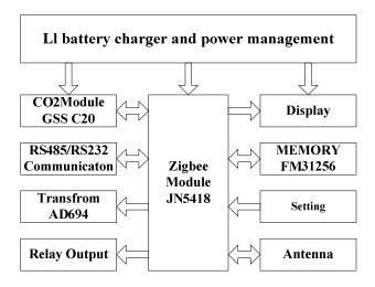
Fig. 3. Hardware design structure
