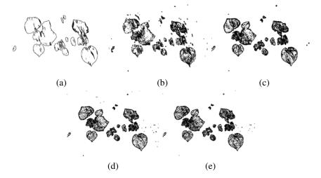
Fig. 7. Blurred cotton image and 4 kinds of algorithm recovery image after contour extraction
