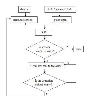
Fig. 2. CPLD Work Logic Flow Chart
