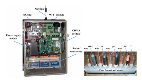
Fig. 1. The water-quality dynamic monitoring system
