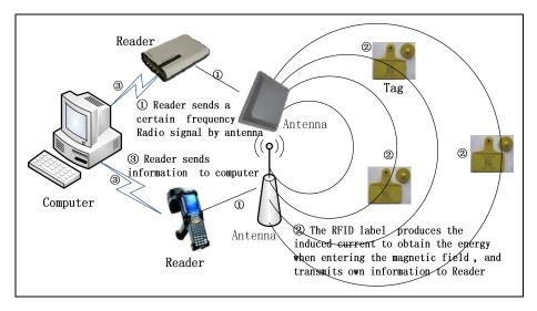
Fig. 3. The scheme of RFID applications
