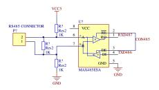
Fig. 4. RS485 Communication Module
