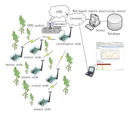
Fig. 1. Overall system architecture of the web-based remote sensing network
