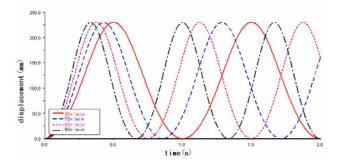
Fig. 3. The displacement curve of centroid of blade at 60~90r/min
