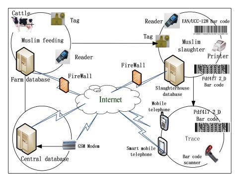
Fig. 1. Overall structure of system
