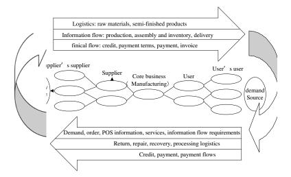
Fig. 2. The logistics, information flow and finical flow of supply chain
