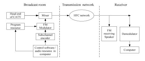
Fig. 3. Work flow of cable addressable broadcast
