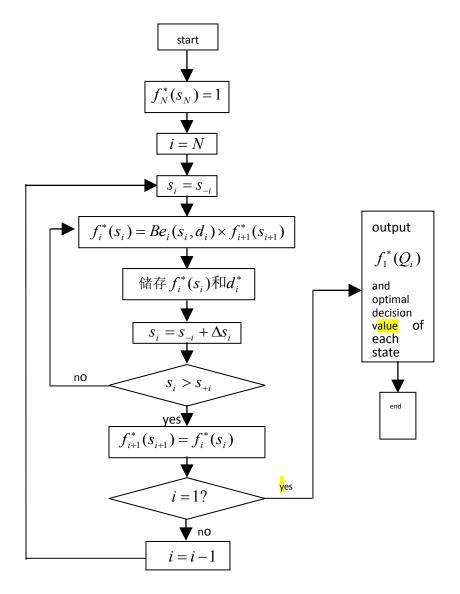
Fig. 2. Program of reverse algorithm of dynamic planning
