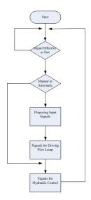
Fig. 7. Software-Control Flow Chart of Controller
