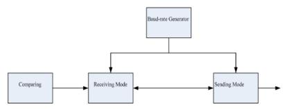
Fig. 8. Basic Principle Diagram of UART
