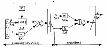
Fig. 1. The picture of GRNN net's conformation
