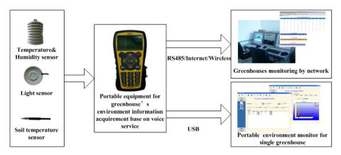
Fig. 1. Structure of portable equipment for greenhouse's environment information acquirement base on voice service
