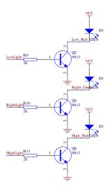
Fig. 6. Position-Pilot-Lamp-Driving Circuit
