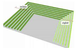
b. The 3D TIN model of inner dump and stope
