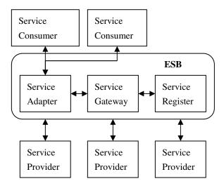
Fig. 4. Enterprise Service Bus architecture
