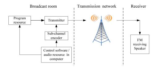
Fig. 4. Work flow of wireless addressable broadcast
