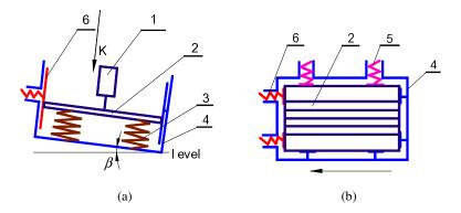
**Fig. 1.** A model of a soil-tuber separation device: (a) front view; (b) K direction view except the linear motor .1-linear motor; 2-rectangular screen; 3- supporting springs; 4-frame; 5-dampers; 6-dampers. Arrow denotes direction of travel.
