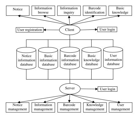
Fig. 1. System structure of TBIS
