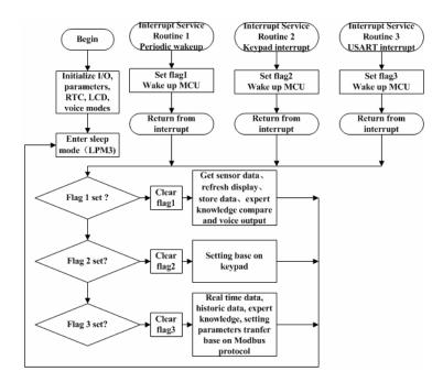
Fig. 4. The structure of low power software
