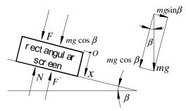
Fig. 2. Forces acting on a rectangular screen in vibrating direction
