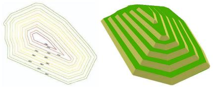
a. The designed 2D vector model of dump b. The designed 3D TIN model of dump
