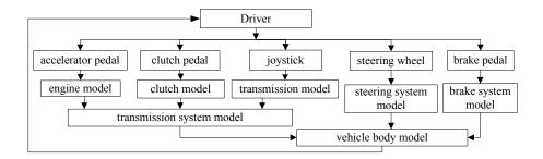
Fig. 6. Closed-loop of tractor dynamic model
