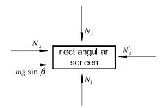
Fig. 3. Forces acting on a rectangular screen at the plane perpendicular to the vibrating direction
