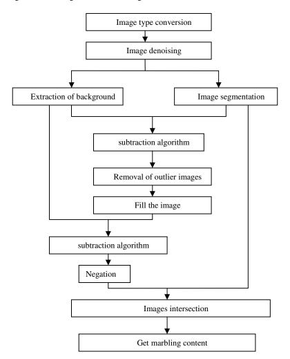
Fig. 2. Flow chart of image feature extraction
