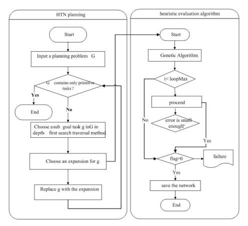
Fig. 3. Heuristic Intelligent Planning Algorithm
