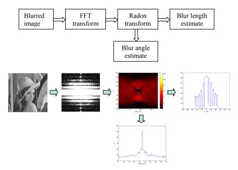
Fig. 1. The process of finding blurring parameters
