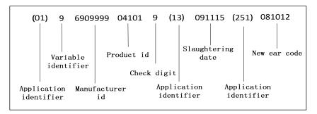
Fig. 4. Encoding Structure of EAN/UCC-128
