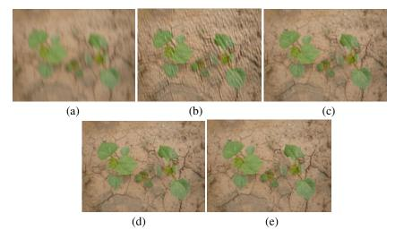
**Fig. 5.** Blurred cotton image and recovery image by 4 kinds of algorithms, (a is blurred cotton image, b is image recovered by Blind Algorithm, c is image recovered by L-R algorithm, d is image recovered by Reg algorithm, e is image recovered by Wiener algorithm)
