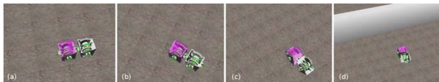
Fig. 13.6 Evolved motion of two joined robot modules in the projects’ ‘Symbricator Simulator’. The hinges of the two modules are contracted in an oscillations by the evolved AHHS. This pushes the organism forward.
