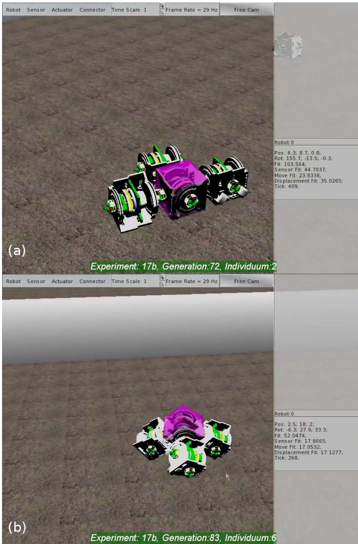
Fig. 13.8 Two different motion patterns evolved successively with the same body shape. a: flat body, oscillators move peripheral hinges like fins. b: erected posture of the organisms, peripheral robots moved like legs.
