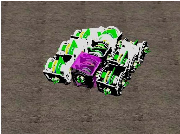
Fig. 13.1 Exemplary configuration of 9 robots arranged and coupled in a 3 \times 3 layout in our proposed EMMR approach. The process that is able to form this body shape from a swarm of autonomously moving single robot modules has to be evolved. Artificial evolution should then also generate controllers that are able to move this robotic organism in a self-organized way. Multiple feedback loops, that allow self-organization to work at specific points of control, is proposed to enhance and support artificial evolution.
