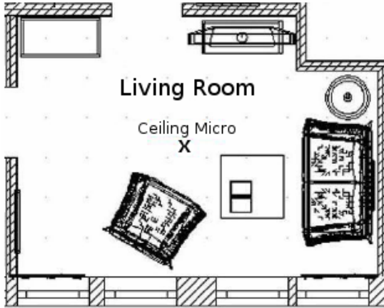
Fig. 5. Layout of the acoustic environment in the living lab. The position of the ceiling microphone, which is used for the experiment, is indicated by an ‘X’. The armchair in the bottom centre of the room indicates the position of the speaker.
