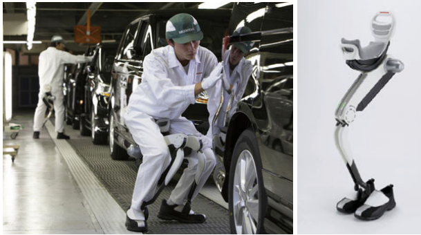
Fig. 7. Honda began its researches regarding electronic assistants in 1999, with the purpose to help older and weaker people or factory workers who have difficulties with walking. Honda.
