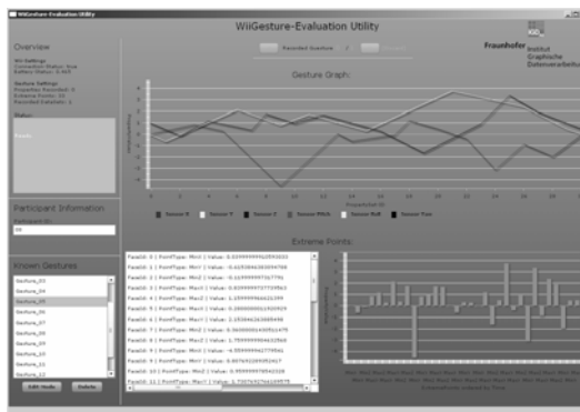
Fig. 2. Screenshot of the Evaluation-Tool, which stores the data from the accelerometers of the WiiMote to performed gestures by a participant.
