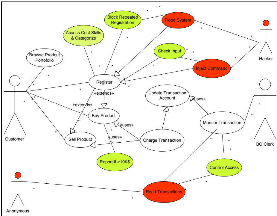
Fig. 4. Use Case model extended with "Security Use Cases"
