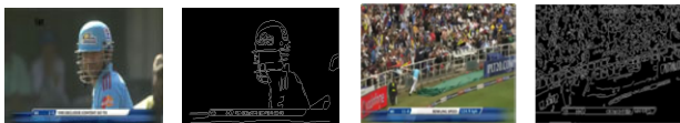
Fig. 6. (a) Close up image. (b) Edge detection results of fig.(a). (c) Crowd image. (d) Edge detection results of fig. (c).
