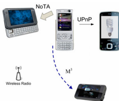
Fig. 4. Audio rendering services in an internet tablet and a Symbian OS Smartphone controlled by input services on a mobile phone established using the three distinct service interconnect approach
