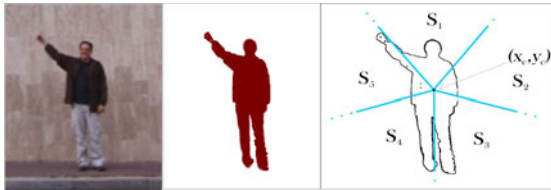
Fig. 3. Model-based 17-dimensional Feature set
