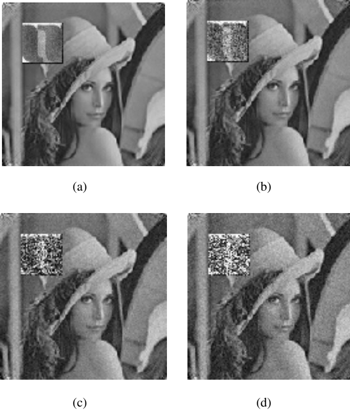
Fig. 8. Extraction of watermark with addition of Noise in Watermarked Image having value for mean( m ) and standard deviation ( s ): (a) m=0 , s=1 ; (b) m=0 , s=10 ; (c) m=0 , s=50 ; (d) m=0 , s=100
