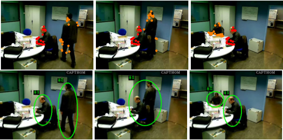
Fig. 1. Illustration of tracking result with a partial occlusion. First row: input images with interest points associated with each object, second row: tracking result.
