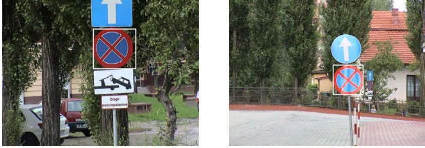
Fig. 5. Examples of correct classification of the signs despite the imprecise detection and under different color and/or lighting conditions. In all cases the color images were converted to the monochrome versions by taking exclusively the blue channel. Then intensity values were conditioned by histogram equalization method.
