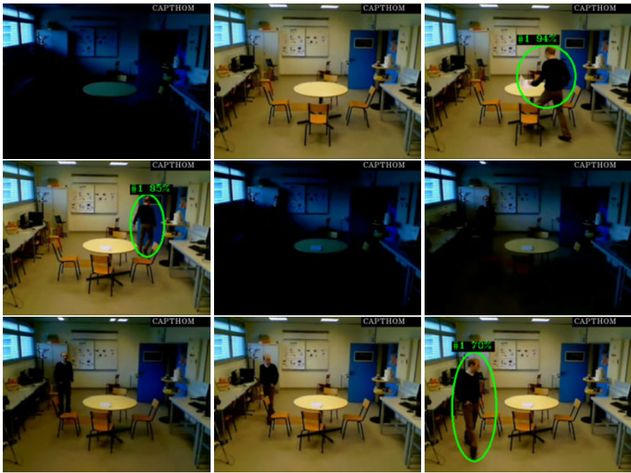
Fig. 5. Example of results obtained with the CAPTHOM method on a video presenting illumination changes
