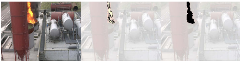
Fig. 2. Source frame, detected blocks with high energy threshold, and corresponding component with lower energy threshold
