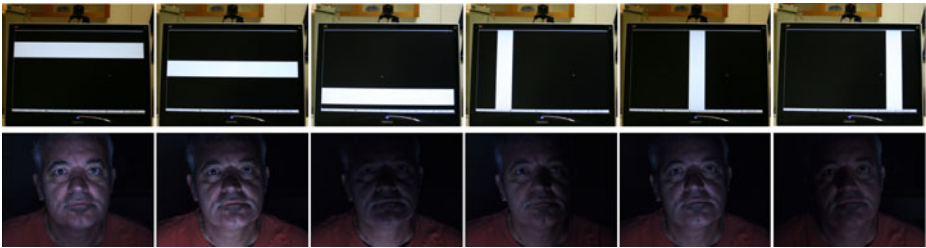
Fig. 1. Multiple images of a subject are acquired while illumination is varied by moving a white stripe on a computer screen
