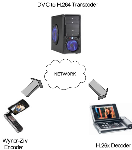
Fig. 1. System using a DVC / H.26X transcoder
