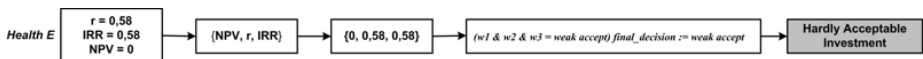
Fig. 4. Example UBMSS system for analysing and assessing the acceptability of an investment
