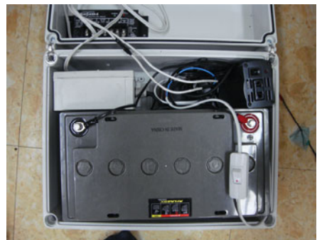
Fig. 8. salinity sensor receiver, integrated battery
