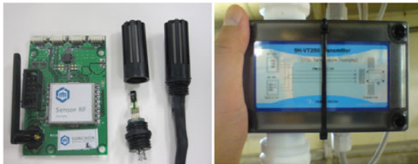
Fig. 2. Integrated sensor node and CO2 sensor
