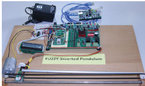
Fig. 16. Fuzzy Inverted Pendulum example on LAB-PIC
