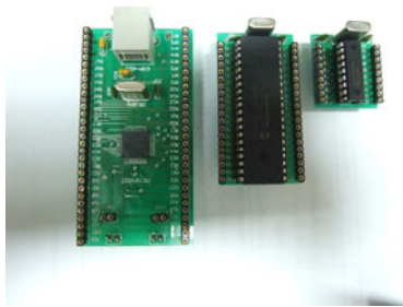
Fig. 13. PIC chip example that is in the kit ( PIC18F6627 )
