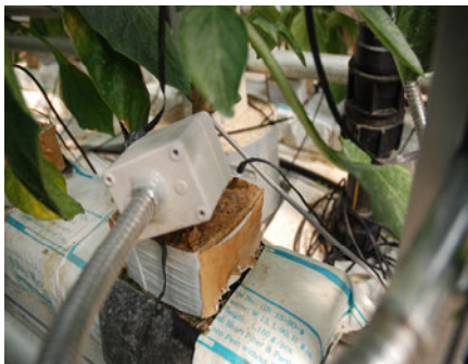
Fig. 10. Root Zone Sensor
