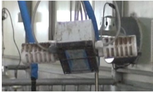
Fig. 5. Plastic box to protect the sensor node
