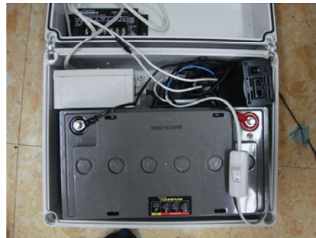
Fig. 8. salinity sensor receiver, integrated battery
