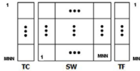
Fig. 1. Individual representation of an ANN. Note that TC represents the topology of the network, SW represents the synaptic weights and TF represents TF of each neuron.
