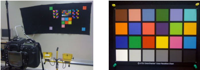
Fig. 2. The image acquisition system, source illuminants and the Munsell ColorChecker Image Reproduction Target chart
