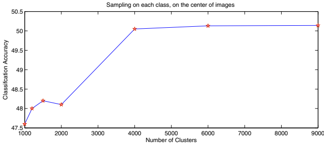
Fig. 4. Creating the dictionary of features from the center of images rather than the whole image
