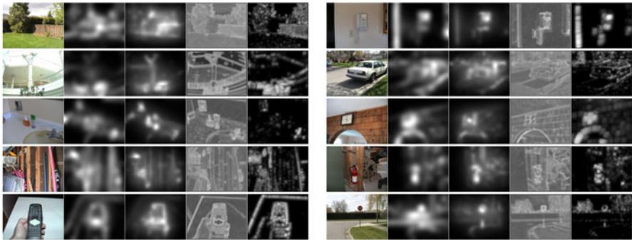
Fig. 2. Input images from [4], then salient regions detected by Itti, GBVS, AIM and CA algorithms
