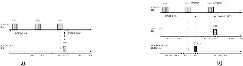
Fig. 1. FrameComm and FrameCommDM communication mechanism
