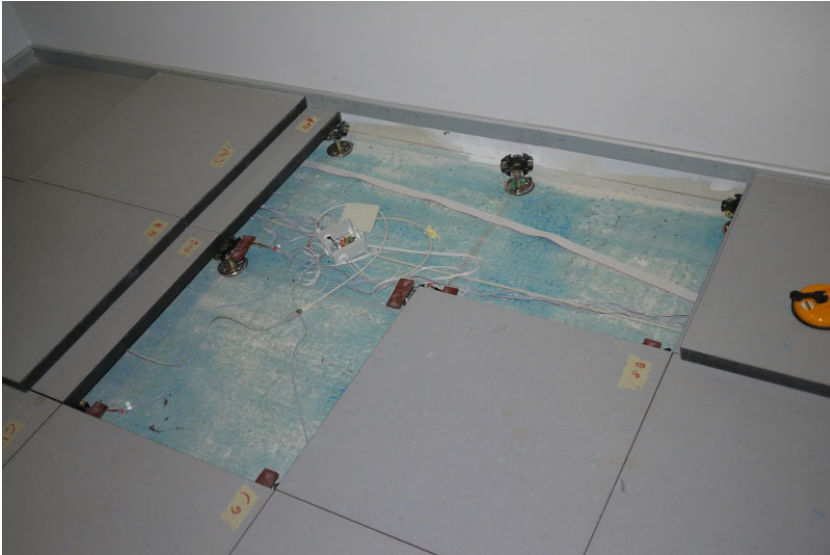
(b) Load sensors attached to iSense node.
