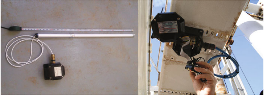
Fig. 2. TelosB motes in ATEX Boxes and 9dB Antennas
