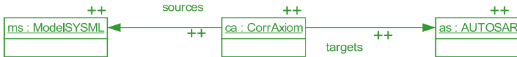
Fig. 8. Axiom of the triple graph grammar for the transformation from SysML to AUTOSAR
