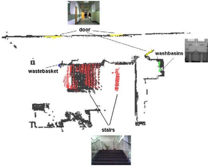
Fig. 18. A top-view of a sample global map of the environment. Cells represent unidentified and identified obstacles, floor and ceiling on the image are omitted.
