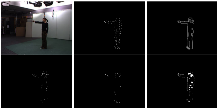
Fig. 2. Comparison of interest point operators. (a) shows a sample frame from a video of a person pointing. The next five images show the feature points selected by: (b) Harris corner detection, (c) Canny edge detection, (d) the scale-space extremal point interest operator of SIFT, (e) Algebraic corner detection, and (f) Fast Radial detection.
