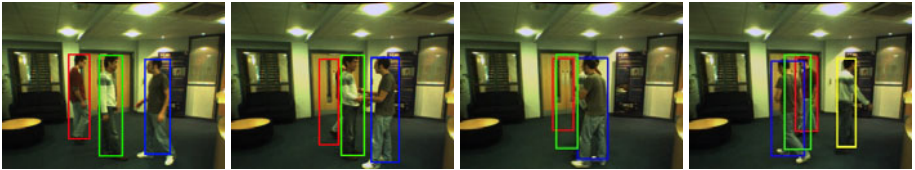
Fig. 10. Tracking results of the mean shift algorithm proposed by Porikli and Tuzel [17]. The frame numbers are 20, 30, 43, and 54, from left to right, respectively.
