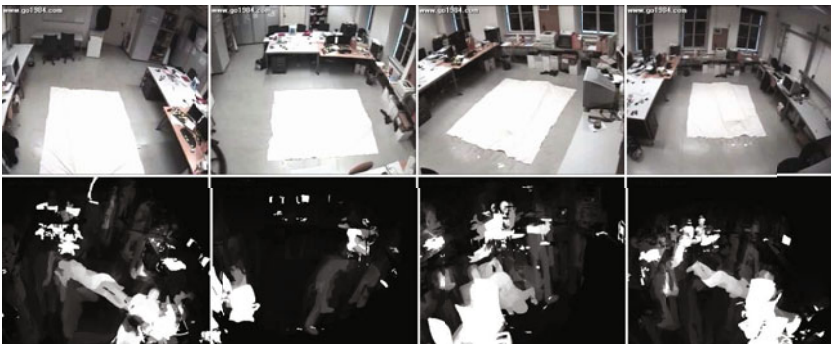
Fig. 3. Four camera views (top row) and the corresponding trained hitmaps (bottom row)
