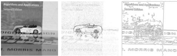
Fig. 2. Examples of occluding contours achieved by the OC-Cam system. Left: original normal images. Middle: corresponding OC images. Right: result of Canny edges [5] for comparison.
