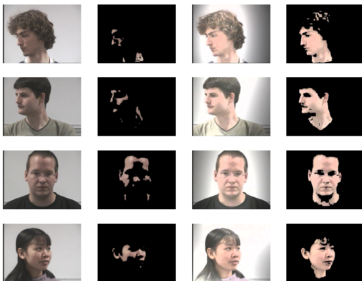
Fig. 5. Face segmentation examples. In the first and second columns are shown the original images, and their respective segmentation results. In the third and fourth columns, are shown images after the application of our shading attenuation method, and their respective segmentation results.
