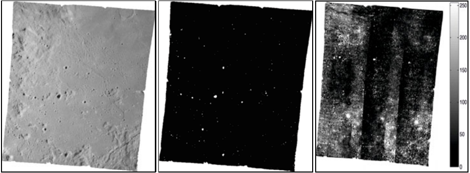
Fig. 5. Orbital image: (left) input image, (middle) binary shadow map with shadow regions shown in white, (right) DEM confidence map (brighter areas have higher estimated error)
