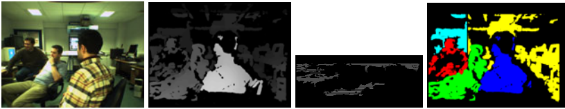
Fig. 1. Depth-based segmentation. (left to right) The input left colour frame, The Disparity map, The Depth density image, Depth-based object detection.
