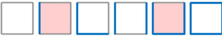
Fig. 6. Configurations of degenerate pairs in a unit square. A pair of tensor samples is drawn in blue if it is degenerate, and the square is shaded in red if it contains a degenerate point.
