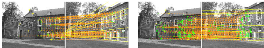
Fig. 7. Lewven Castle : two distant images from M. Pollefeys' sequence. Left: ASIFT. 94 matches, only among points from the same façade. Note that repeated windows yield false correspondences with the fourth window in the second image (which is not present in the first one.) Right: I-ASIFT+F. 118 matches (24% are not nearest neighbours), distributed over the whole building. Except for two, all of them are correct. The fundamental matrix is then estimated over the retrieved set of correspondences. The epipolar lines (in yellow in the right images) corresponding to some handpicked points (from the left images) prove that I-ASIFT permits to reliably estimate the camera motion. The points associated to the handpicked ones are indeed less than 1 pixel away from the corresponding epipolar line. In contrast, the camera motion cannot be retrieved from ASIFT. As a comparison, MSER gives 5 matches, and Harris/Hessian Affine 20-30 matches mainly between wrongly associated repeated patterns. (code from Mikolajczyk et al.'s www.featurespace.org ).
