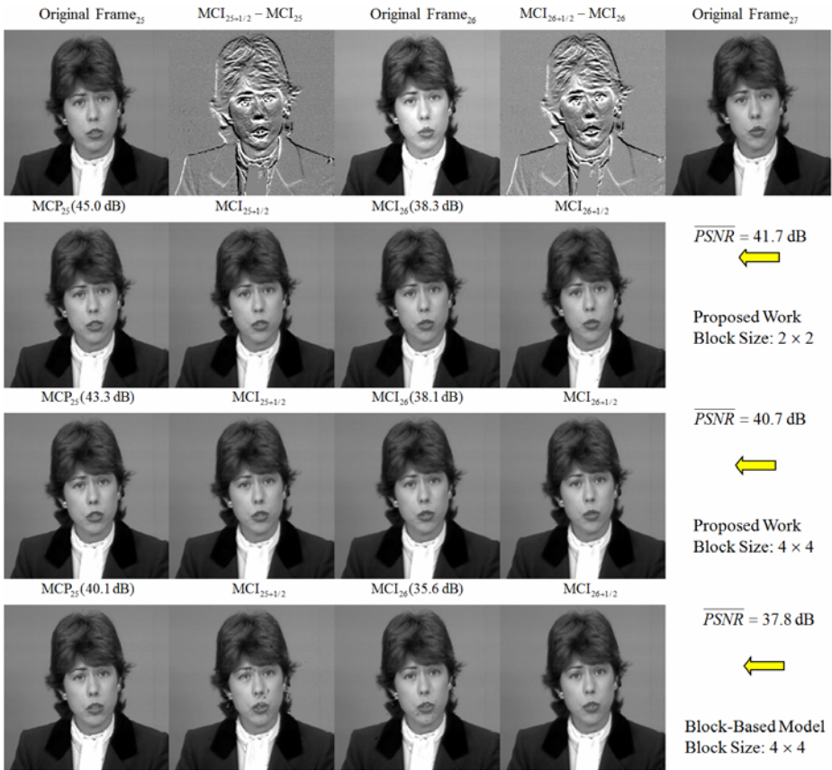
Fig. 3. A Claire image sequence with frame from 25 to 27 ( 196 \times 196 ), the motion fields are estimated by current method and block matching algorithm with different block sizes ( 2 \times 2 and 4 \times 4 ) as the motion estimation parameters, MCP and MCI motion pictures synthesized by the proposed framework [19], and inter-frame difference images of MCI_{25+1/2} - MCP_{25} and MCI_{26+1/2} - MCI_{26}
