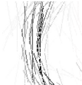
Fig. 2. Illustration of the CFT. The lines illustrate the secondary curve field for the image in Figure 1a. (For clarity, we only plot straight curves.) In this figure, each curve segment is plotted with an intensity that reflects the weight associated with the curve segment. The CFT is computed by at each pixel, summing the weight for each curve segment that intersect the pixel.
