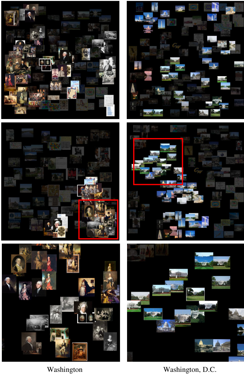
Fig. 1. Comparison between image organization results generated using the visual feature vector alone (top) and the hybrid feature vector (middle), as well as the zoomed-in views of the areas marked by the red squares (bottom). For illustration purposes, images of several persons related to George Washington are highlighted in the left dataset, and the ones related to buildings in Washington, D.C. are highlighted in the right dataset. One can readily see that the grouping of the highlighted images is much better with the hybrid feature vector (middle) than the visual feature vector (top).
