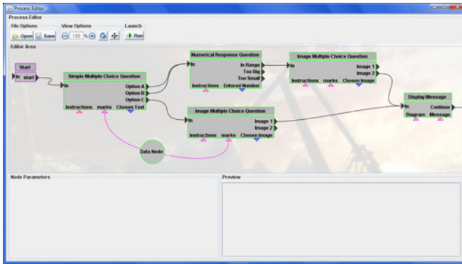
Fig. 3. A Sample Question in which the problem branches into two possible correct paths to the solution. The green colored box-shaped nodes represent Question Nodes whereas circles represent data nodes.
