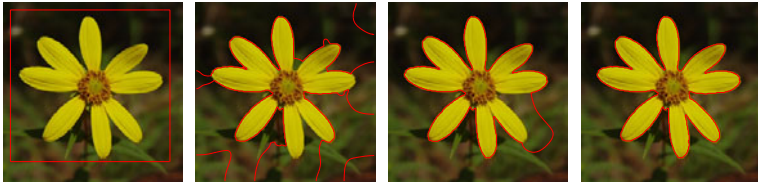
Fig. 5. The result of our method for a color image of flower. It shows the curve evolution process from the initial contour to the final contour.
