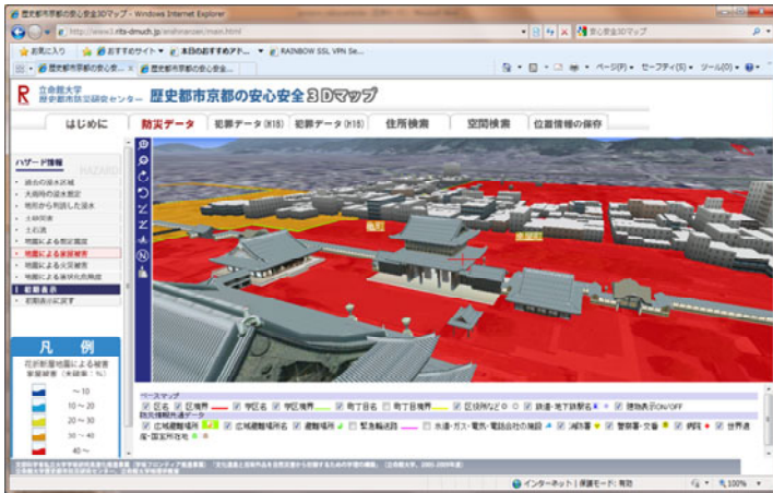
View of building collapse risks caused by a possible earthquake (Hanaore fault) around Higashi-Honganji temple
