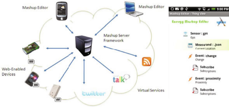
Fig. 2. Architecture of the physical mashup framework and screen-shot of a mobile mashup editor
