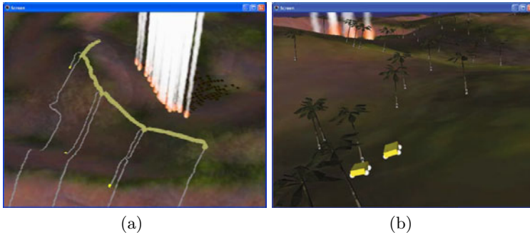
Fig. 4. (a) Four robots creating a firebreak. (b) Detailed view of mobile robots moving to the fire.
