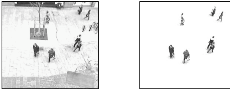
Fig. 3. Raw image (left) and the same image after background subtraction (right)
