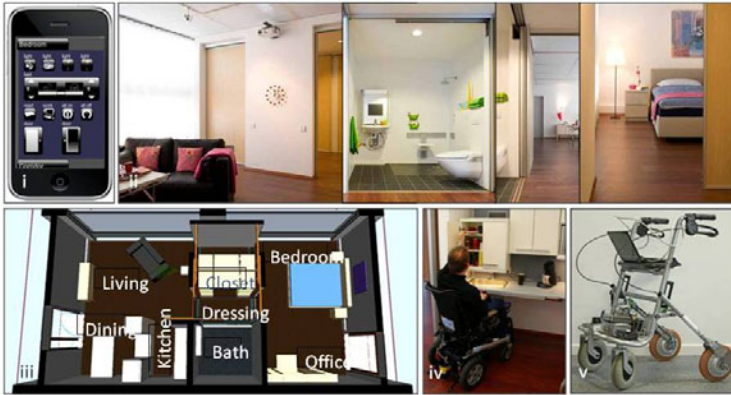
Fig. 2. Demonstrators at the BAALL: (i) remote rontrol on iPhone; (ii) instrumented flat; (iii) synchronized virtual 3-D model; (iv) autonomous wheelchair; (v) intelligent walker (photos © raumplus)
