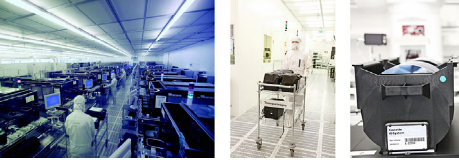
Fig. 2. Left: Clean room in a semiconductor factory; Center: Operator moving lot boxes ; Right: An open lot box with wafers
