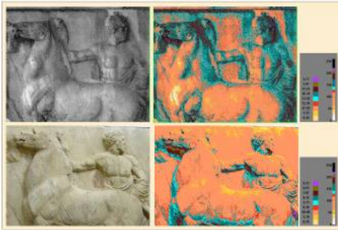
Fig. 11. Pictorial and digital images of the West Frieze - Block III before and after laser cleaning treatment
