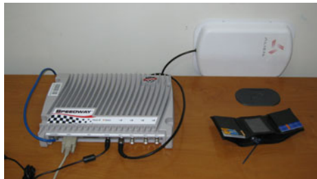
Fig. 2. WISP tag inside of a wallet in front an Impinj RFID Reader
