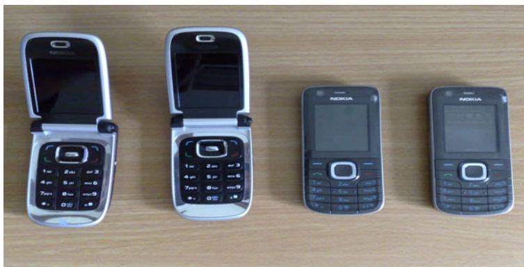
Fig. 2. Devices used in the relay attack – Device B (Nokia 6131 NFC), Proxy A (Nokia 6131 NFC), Proxy B (Nokia 6212 Classic NFC) and Device A (Nokia 6212 Classic NFC)
