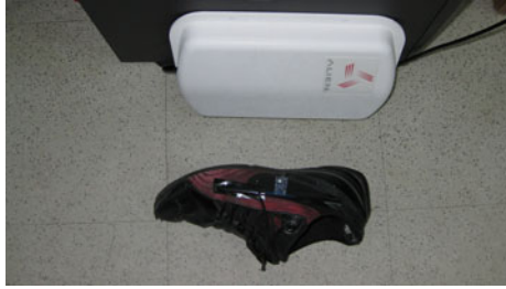
Fig. 3. WISP tag fastened to a shoe in front of an Alien Antenna connected to an off-camera Impinj RFID Reader
