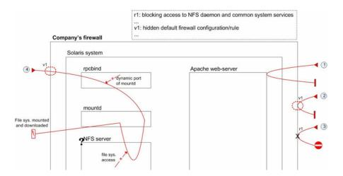
Fig. 2. MUCM for the (part of) penetration test example from the experiment
