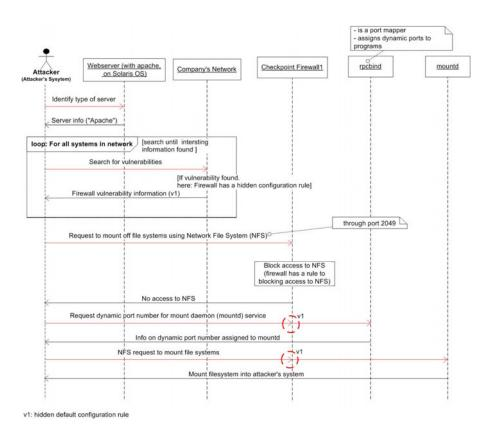
Fig. 4. MUSD for the (part of) penetration test example from the experiment
