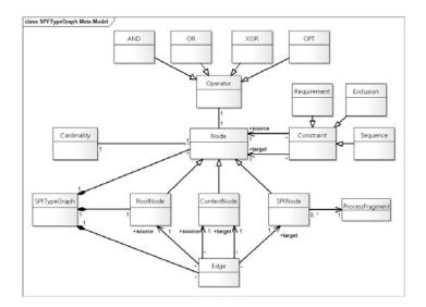
Fig. 3. Meta model of SPF type graphs as UML class diagram
