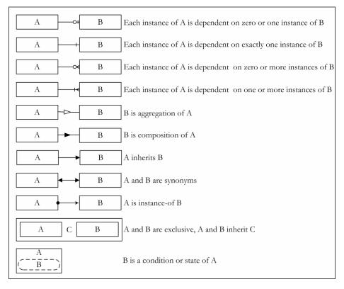
Fig. 1. Representation of static dependencies, structural aspects, in EM (adapted and modified from [16])
