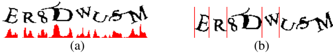
Fig. 6. (a) Vertical pixel histogram, (b) segment five blocks (Both Images are taken from [10])
