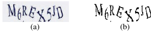
Fig. 5. (a) Original image, (b) Binarized image (Both Images are taken from Microsoft CAPTCHA)
