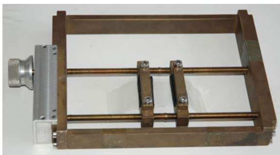
Linear Dichroism Spectra - Measurement, Fig. 2 A mechanical film stretcher showing oppositely threaded screws to ensure even stretching of the film
